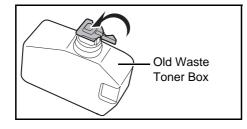
3 Close the cap to the old waste toner box after removing the box from the machine.
